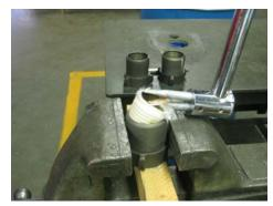
remove the ring. Overdriving the point into a small diameter coupling may drive it in too deep and puncture the bottom of the coupling bowl.
